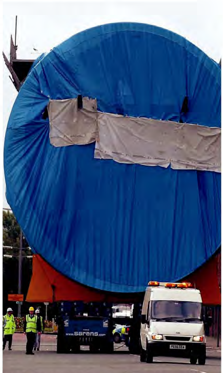
CLUES: This shows a hull section of the Astute-class submarine Audacious on its way to the Devonshire Dock Hall in 2010. See if you can find the 12 words linked to submarines we have hidden in the wordsquare
