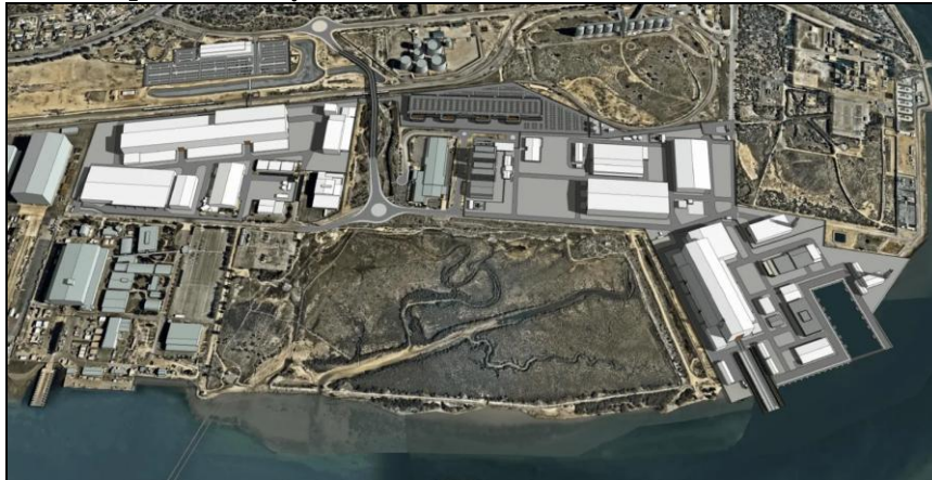
(Left) Area 1 – main fabrication hall and production facilities (Centre) Area 2 blast and paint workshops (Right) Area 3 consolidation hall, ship lift and graving dock (Image: ANI).
